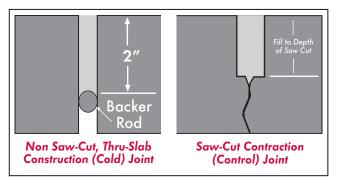
In construction (formed) joints that are not saw-cut, **Spal-Pro RS 88** should be installed at a minimum 2" depth. **DO NOT USE COMPRESSIBLE BACKER ROD IN STANDARD SAW-CUT CONTRACTION/CONTROL JOINTS!** Rod
