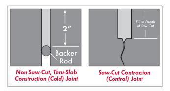
In construction (formed) joints that are not saw-cut, **Edge-Pro 90** should be installed at a minimum 2" depth. **DO NOT USE COMPRESSIBLE BACKER ROD IN STANDARD SAW-CUT CONTRACTION/CONTROL JOINTS!** Rod may be used 2" down in construction or saw-cut joints exceeding 2" in depth ONLY.
